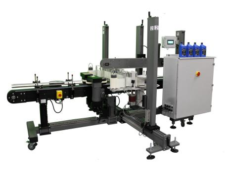
The 625 is a heavy-duty, affordable front-back labeling system. The compact size, durability, and low cost make the system ideal for small, medium or long-run jobs. Large volume, high-speed packing applications are handled with ease.
